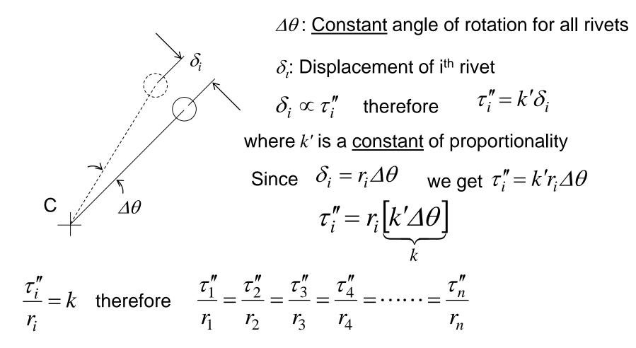
Note that farthest rivet from C experiences the largest secondary shear stress
