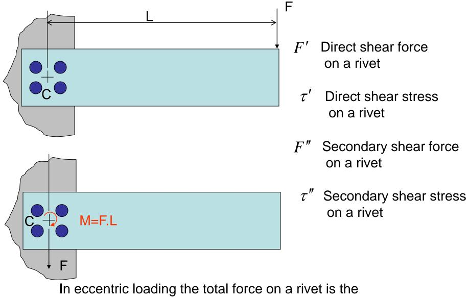
superposition (vector sum) of direct and secondary shear forces.
