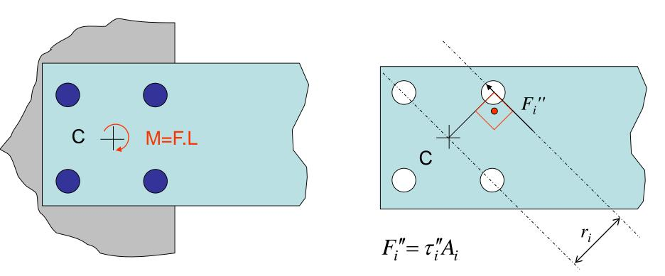
Secondary shear force on i<sup>th</sup> rivet,  $F_i$ '' is perpendicular to the line joining the centroid of the rivet group and the center of the rivet. The distance between the centroid C and center of i<sup>th</sup> rivet is  $r_i$ .
