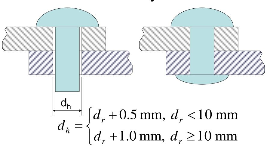
•When the bottom head is formed, rivet shank expands and fills the gap.
